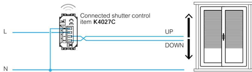
For correct operation, connect also the neutral conductor to the connected devices.
